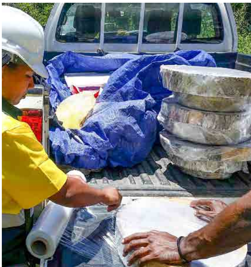
Wrapping of Maesopsis Density discs for density analysis
