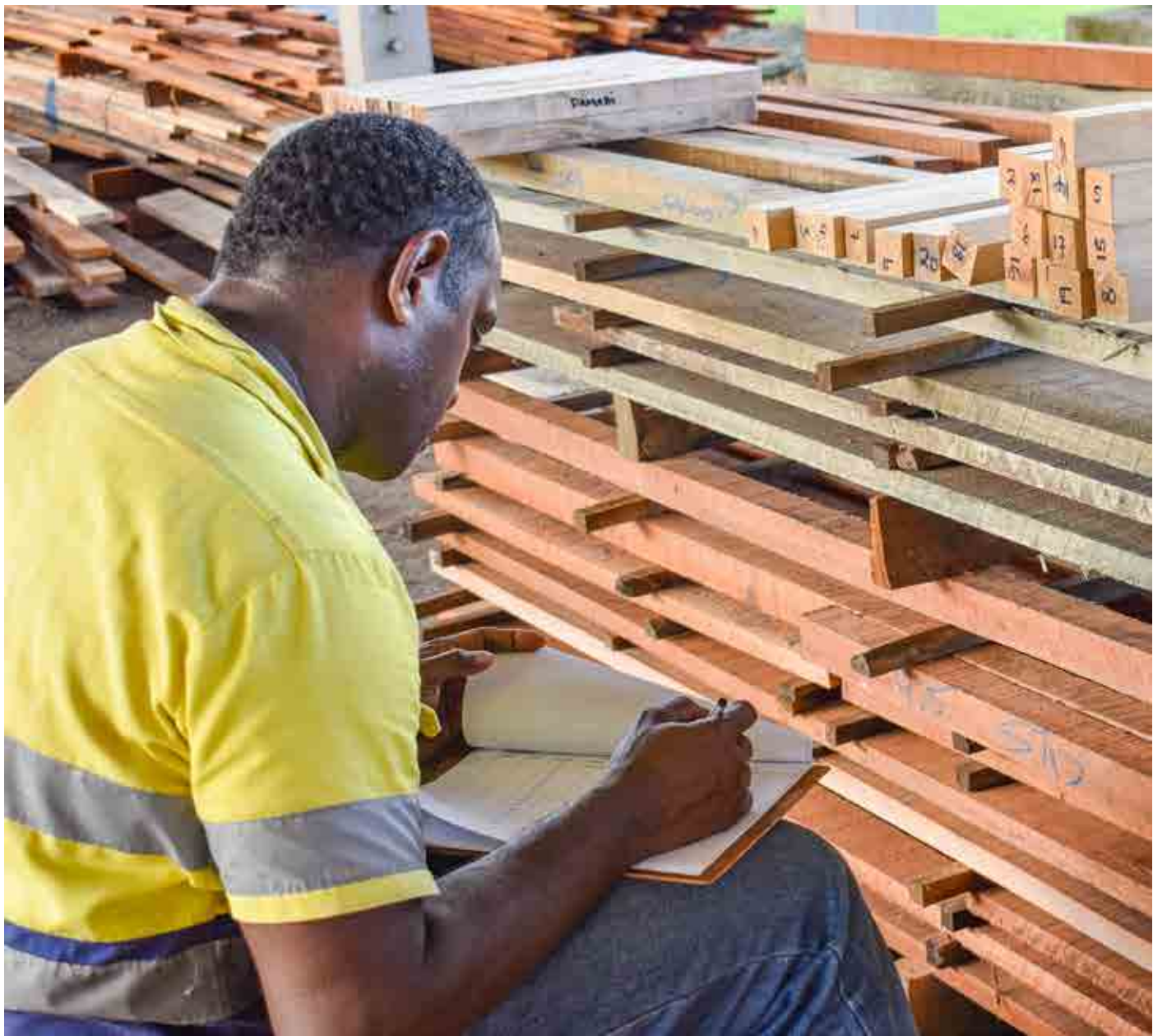
Grading of timber stakes before instalation in research trial sites.
