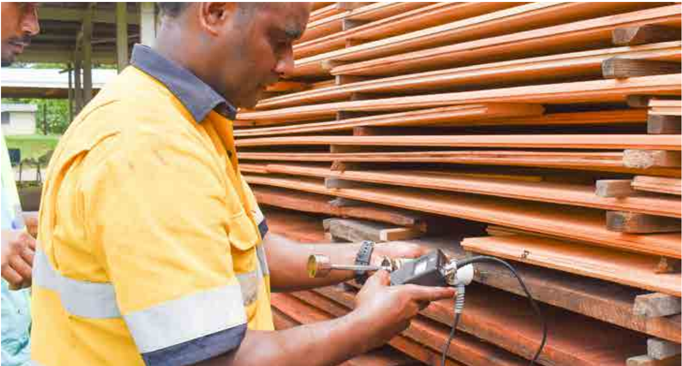
Moisture content assessment for kiln dried timbers
