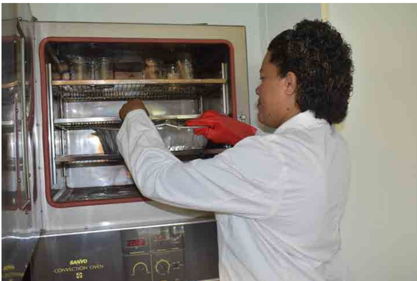
Drying of timber samples for laboratory analysis
